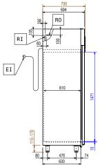
Electrical inlet (power) Refriaerant Inlet Refrigerant Outlet
